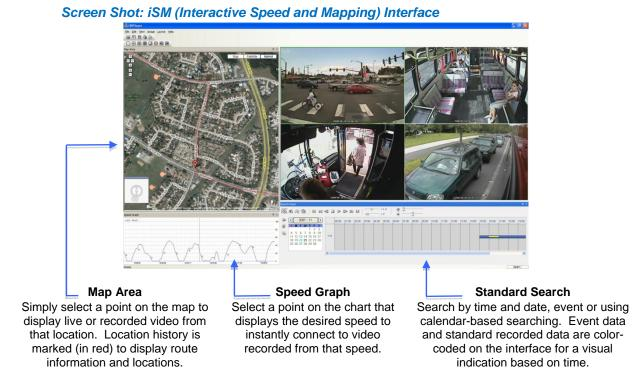
**High Quality Recording:** The RoadRunner™ system uses state-of-the-art H.264 or MPEG-4 video compression providing the highest possible quality video with the longest on-board recording duration. Triplex operation allows for simultaneous recording while providing user live viewing, archiving and system administration functions.
