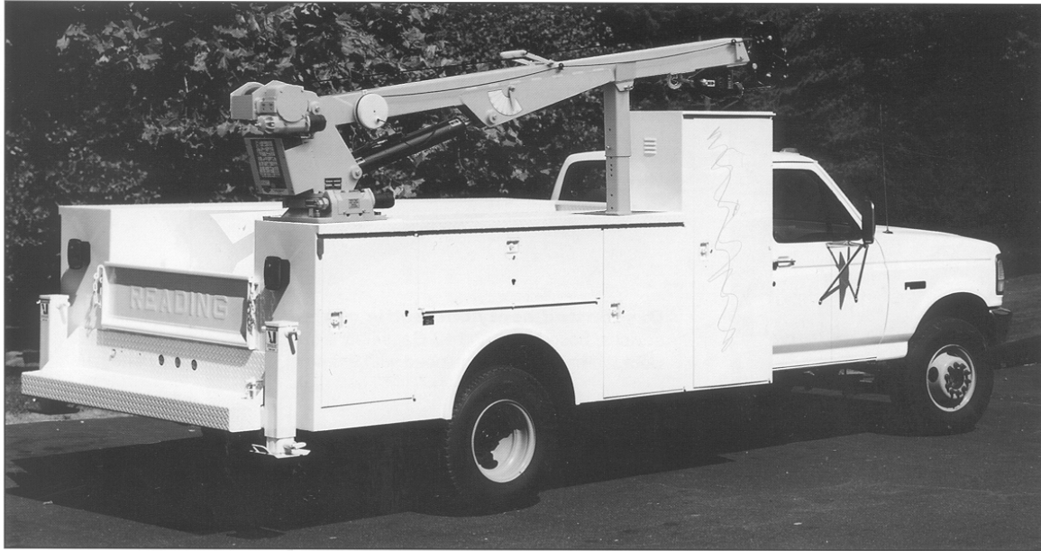
Model shown features optional manual out / crank down outriggers
